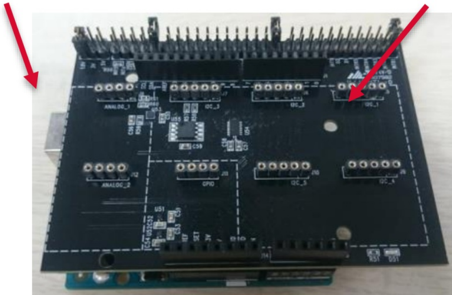
Figure 3. Connection between the Arduino and the SensorShield
