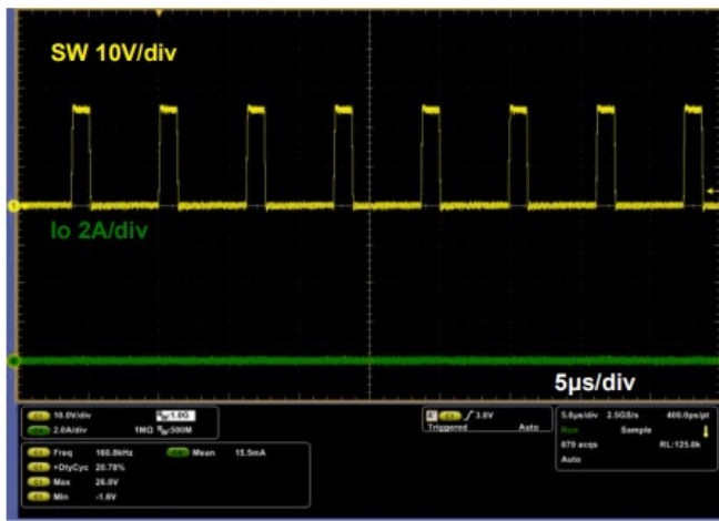
Figure 11-12. Switching Waveform ( V_{in}=24V , V_o=5V , I_o=0A )
