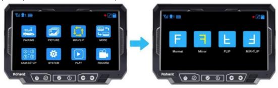
**Tips:** The Screen Rotation Settings can only be switched when the screen is displayed in full screen separately, not in split-screen mode.
