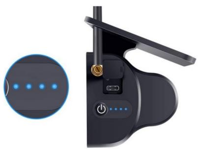
4. Pick up the camera close to the monitor, the monitor appears image means the system is working.
