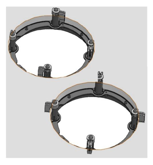
Step 3: Install the baffle to the mounting frame
