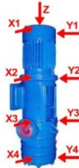
Figure 14: Measuring Points on Machines with Vertical Rotors
