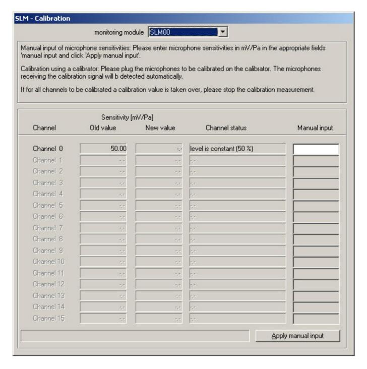
The order you calibrate the microphones does not matter. The microphone with calibrator plugged on is detected automatically by the constant level.
