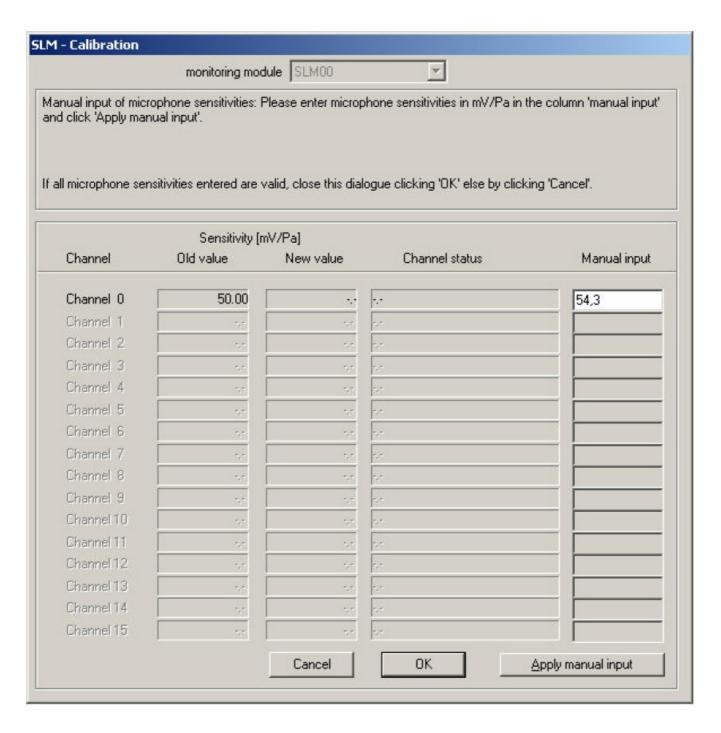
Enter the microphone sensitivities in the column 'Manual input' and click 'Apply manual input'.
