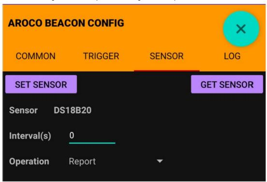
Interval(s): Sensor Reading Interval Range 0,5 to 86400 (Default: 0 – Disable)
