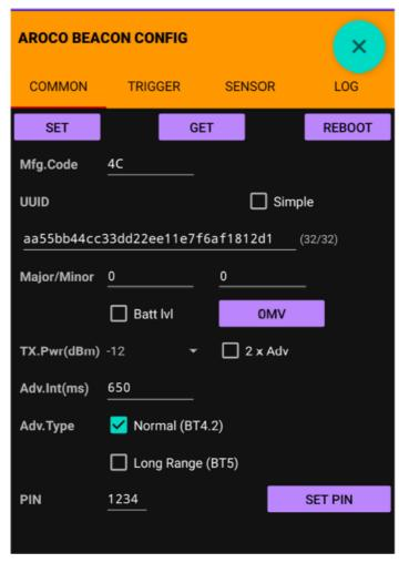
**UUID**: Simple 16 characters in simple (simple check box ticked) or 16 Bytes hexadecimal UUID data can be changed. (Default UUID: aa55bb44cc33dd22ee11+6 bytes Beacon MAC address)
