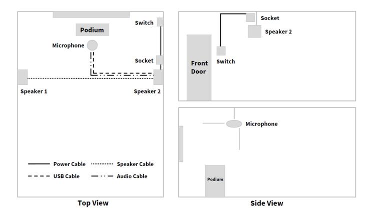
For classroom installation, please refer to the figure below. The USB interface is used as the power supply port of the microphone, and can be connected to the socket or adapter with USB interface. The power supply voltage is DC 5V. The SPK-OUT audio output interface is output to active speakers or power amplifiers through a 3.5mm interface audio cable. It is recommended to use low-latency active speakers first, and the speaker experience will be better.
