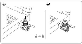
Push the button to lock the device.
