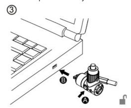
Press the release button and insert the locking tip into the slot.
