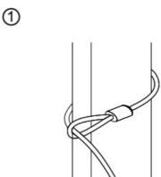
Wrap your cable around an immovable object, by crossing the lock body, through the loop, on the opposite end of the cable.
