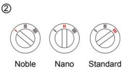
You must adjust the locking tip before inserting the lock into your device.
