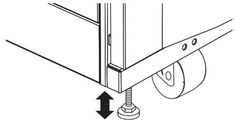
Note: Lower a leveler by turning it clockwise; raise a leveler by turning it counter-clockwise.
