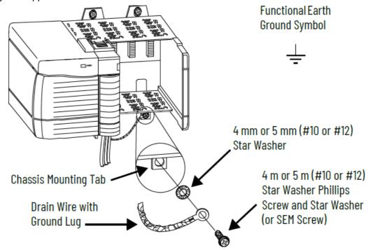
6. When the drain wire is grounded, connect the insulated wires to the field side.
