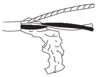
3. Twist the foil shield and drain wire together to form one strand.
