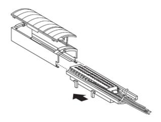
**IMPORTANT** If additional wire routing space is required for your application, use the extended-depth housing, catalog number 1756-TBE.
