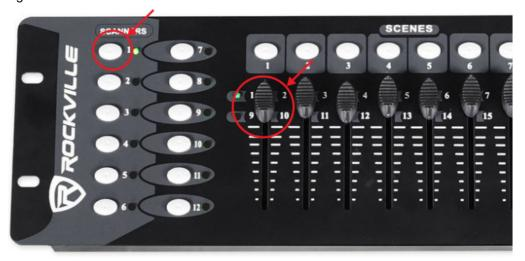
3. To add the scene, press the PROGRAM button for 3 seconds to enter program mode. Now press MIDI/ADD then press the SCENE button for the specific scene. The display screen on the unit will flash indicating that the scene has been added. To add more scenes within that bank, repeat steps 2 and 3. To create additional banks, repeat steps 1-3.
