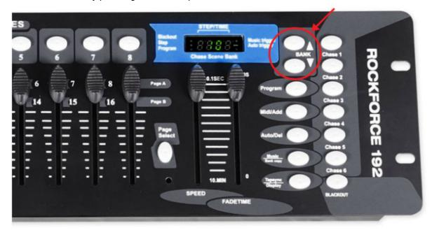
2. Select the desired fixture by pressing the appropriate SCANNER button. Select the color you want for the fixture by using the sliders.
