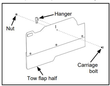
NOTE: For models with (2) hanger mounting locations, secure with additional carriage bolt and nut.
