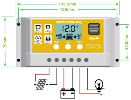
Note: 12V battery with 18V solar panel 24V battery with 36V solar panel
