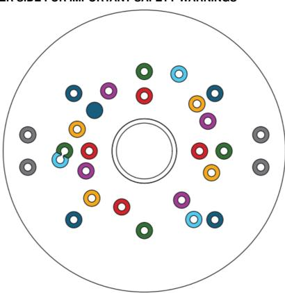
Attach the handles using the included screws through the appropriate mounting holes. Remove the sub-base that came with your compact router and set aside the mounting screws. Locate the correct mounting holes for your router model on the Compact Router Sub-Base with Handles. Align the mounting holes in the Sub-Base with the mounting holes in your router and use the router mounting screws to attach. Center the base following your routers instructions.
