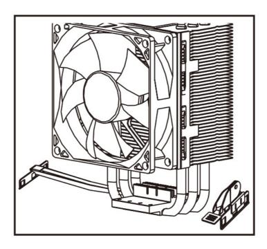
3. Remove the protective cover from the bottom of the cooler, then apply a small dab (about 1/2 the size of a pea) of thermal grease on the surface of the installed CPU. When the cooler is clamped to the processor, the grease will spread evenly to form a thin layer.
