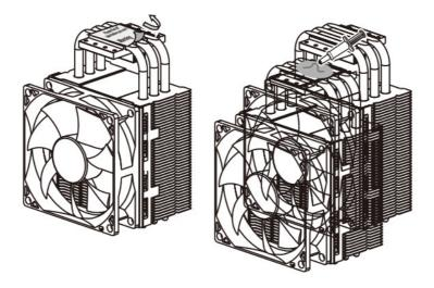
4. Place the cooler on the CPU, then push the lever down to secure the plate.
