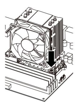
5. Connect the fan power cable. the following graphic is for reference only. Refer to the documentation for your system board for the location of the power connector.
