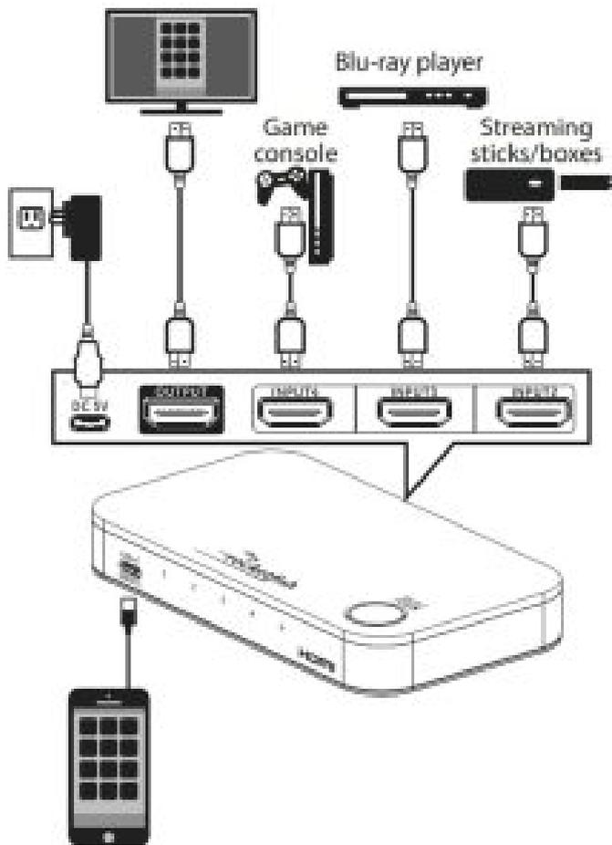
1. Connect up to three HDMI cables and one USB-C cable from your source devices to the switch's INPUT ports.
