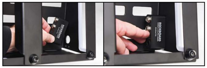
**Step 3**Use the included screws to handtighten the RockBoard® Mini Mounting MOD DC.
