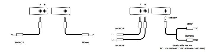
Since the Mini Mounting MOD TRS uses through-connections between the inner and outer jacks, it is also possible to pass signals in the reverse direction to external pedals, such as Wah. Also, by using TRS stereo jacks, "send/return" applications (A- = tip and B- = ring) are easy to realize.
