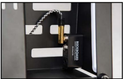
**Step 5**Connect an instrument cable to the outside TRS connector.
