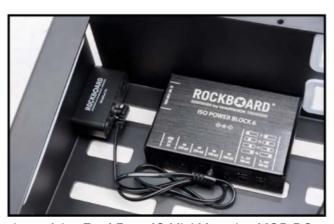
Connect one of the internal sockets of the RockBoard® Mini Mounting MOD DC to the multi power supply.
