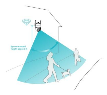
For outdoor use, please install the camera upside down to maximize the waterproof performance and the infrared human body sensor's effectivity.
