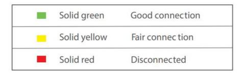
5. If the LED Indicator of a node does not light solid green, relocate it according to the location recommendations in V. part to get better connection.
