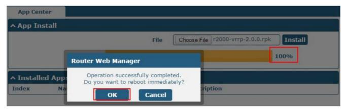
4. After the router is powered on again, log in to the configuration page, VRRP will be included in App Center's "Installed Apps" list, and the function configuration will display in the Services part.
