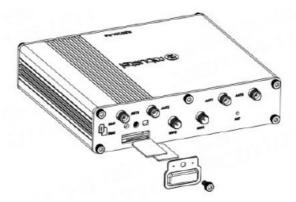
2. Antenna Installation. Rotate the antenna into the antenna connector accordingly.
