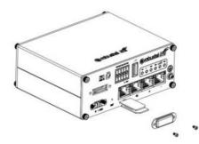
2. Antenna Installation. Rotate the antenna into the antenna connector accordingly. Here take the cellular antenna as example. For 5G 4-IN-1 combo antenna, LHM# cable need to be connected to ANT1 and ANT2 while the MH# cable need to be connected to ANT0 and ANT3. GPS function is available when using the 4 in 1 combo antenna.
