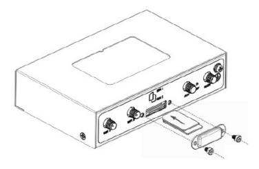
1. SIM Card Installation. Remove the SIM card cover to insert the SIM cards into the device, then screw up the cover.
