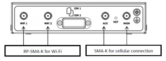
2. Antenna Installation. Rotate the antenna into the antenna connector accordingly.
