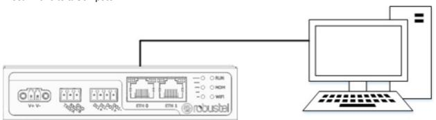
• Connect the gateway's Ethernet port (ETH0~ETH1) to a PC with a standard Ethernet cable.
