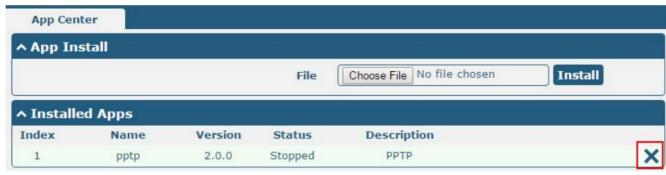
2. Click "OK" in the router reboot reminder pop-up window. When the router finish restarting, PPTP had been uninstalled.
