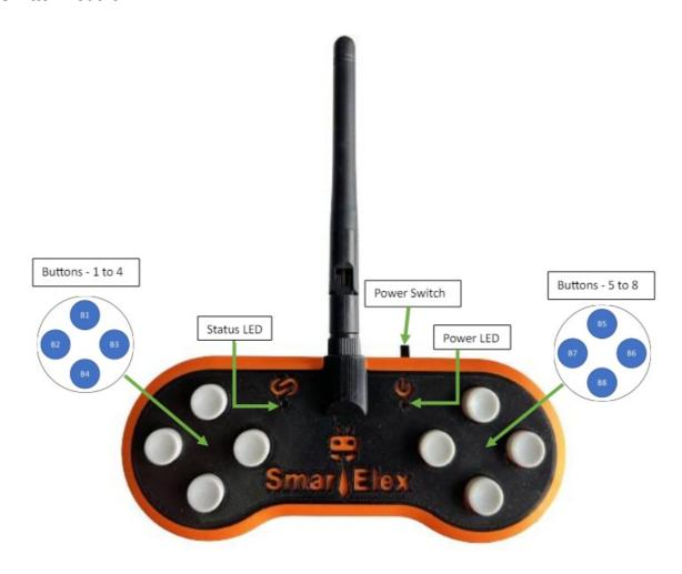
Status LED is always on indicating the transmitter and receiver are communicating with each other
