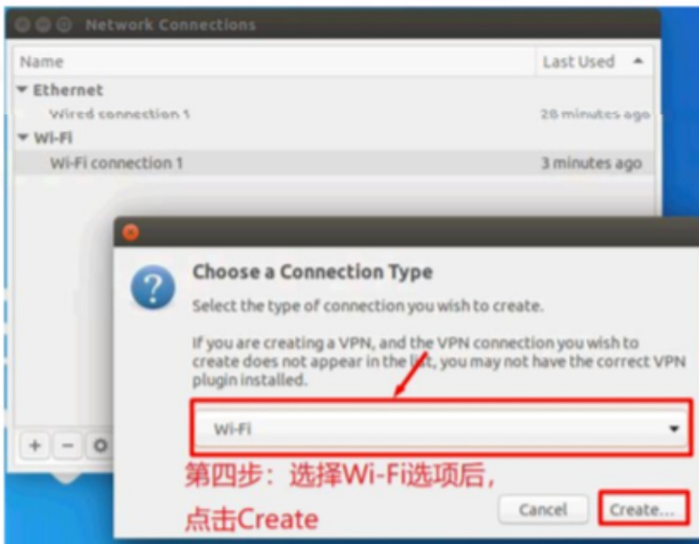
Fig 2-2-3 Jetson Nano Connection to Wifi
