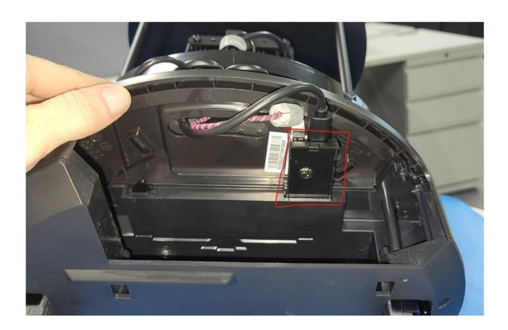
If the cable is correctly connected, you should see a green LED light up on the Rpi card.
