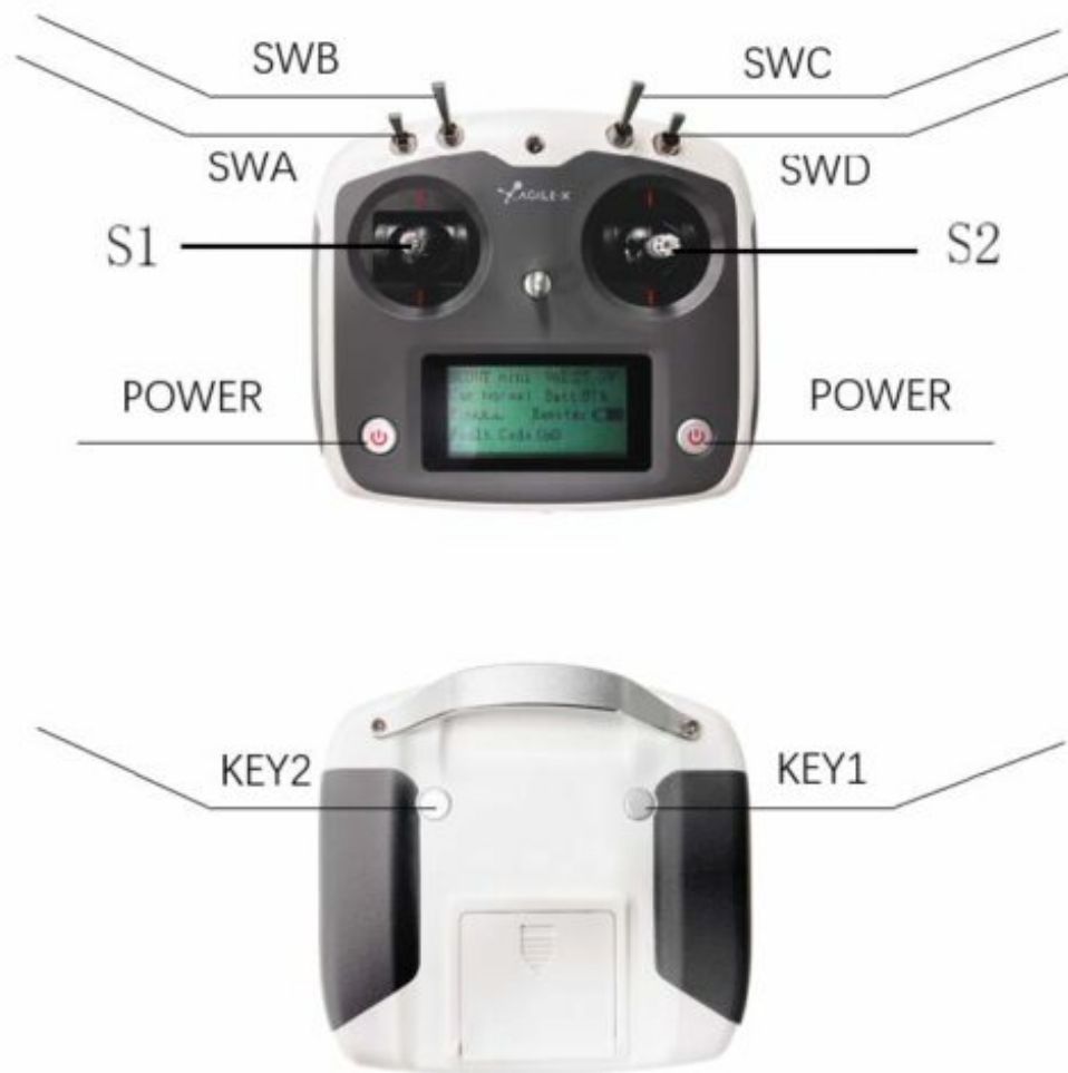
Figure 2.3 Schematic Diagram of Buttons on FS RC transmitter
