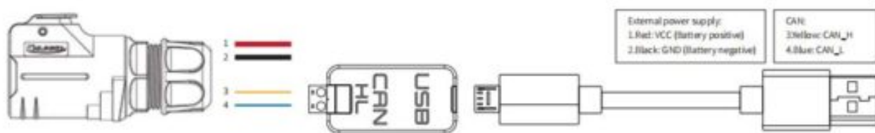
Figure 3.4 CAN connection diagram
