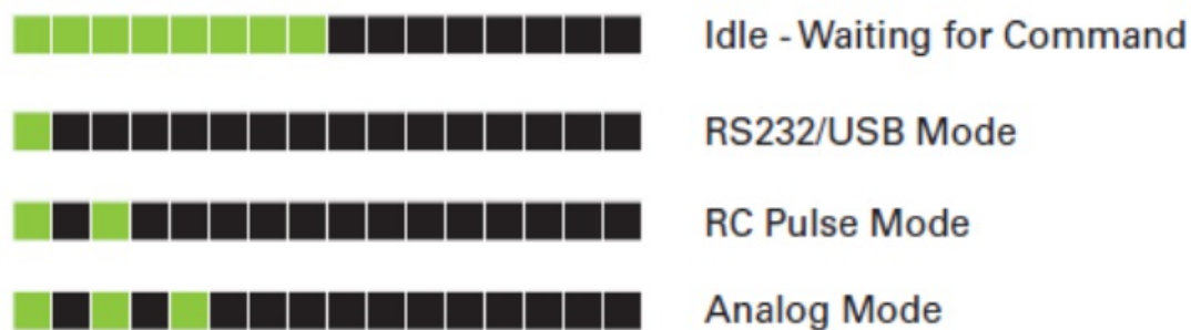
FIGURE 9. Normal Operation Flashing Patterns
