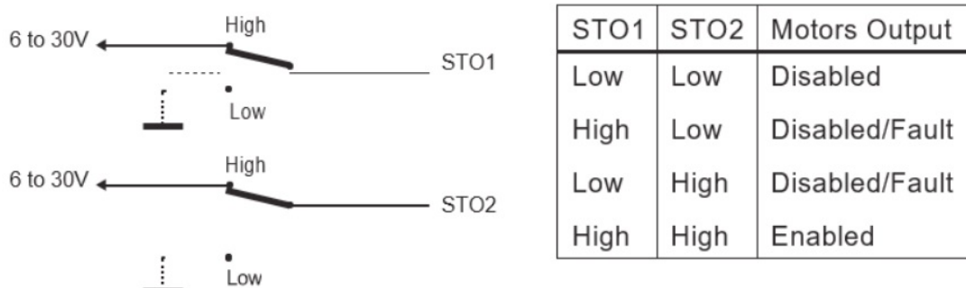
Figure 11. STO input levels effects on controller output
