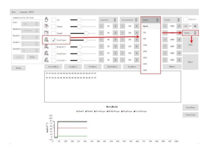
Check the joint to be set, the torque contains 1-1000, here the default power on after 1000.
