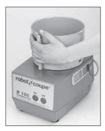
Place the blade onto the motor shaft. Rotate the blade until it drops into place.
