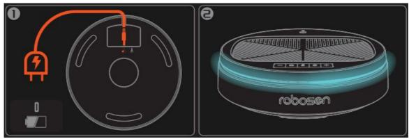
2. Connect the power supply to the robots Plug one end of the robot power cord into the DC charging port on the top of the robosen Al base Lite, and connect the other end to the robot charging port.
