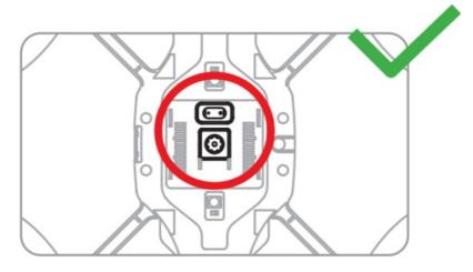
• Drone battery has not expanded and has no signs of structural damage.
