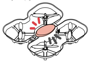
low battery message controller vibration
