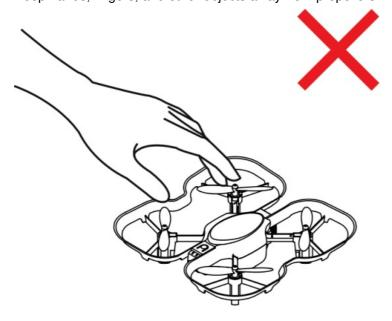
• If the drone crashes, Emergency Stop to shut off motors and avoid motor damage.
