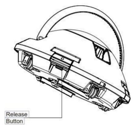
• Once all clips are released, lift the handle to separate the top section of the robot from the base. Remove and rinse the filter net.
