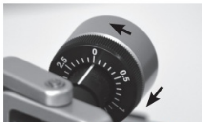
Scale reads zero after setting to 3.0 grams
