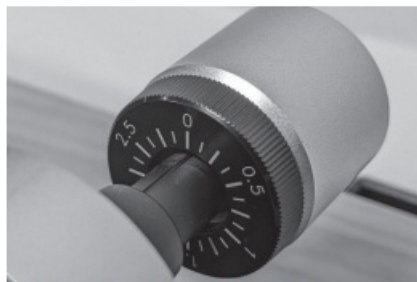
Scale set to zero after balancing the tone-arm
