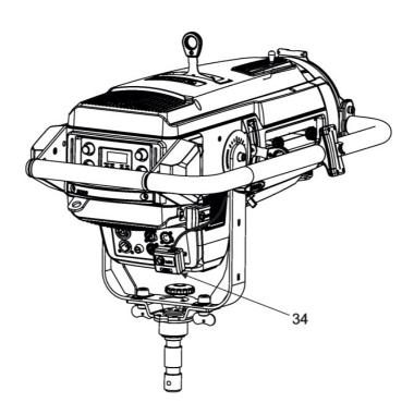
The T11 device can be switched to the FollowSpot mode to make easier control of the fixture with the ROBIN T11 MFS handles installed on the fixture. In the FollowSpot mode, the fixture is controlled by means of four control knobs and the fixture's effects cannot be controlled by DMX.
