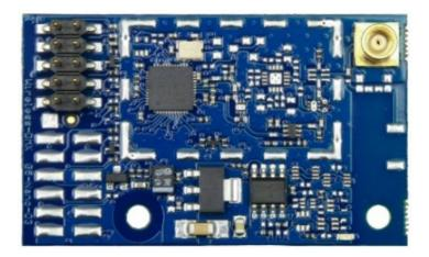
ROBE wireless DMX/RDM module has full support for wireless communication protocols at entertainment market. Modul is based on well known LumenRadio RF technology, with implemented wire interface for connection with Robe products. RF output for MCX interface antenna as standard output.
