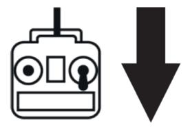
Move the throttle stick to the bottom position within 3 seconds after you hear "Two long and One short beeps" (emitting from the motor) can get you exit the programming mode. The motor beeps "Number" beeps to indicate the number of LiPo cells you have plugged in, and then a long beep to indicate the power system is ready to go.
