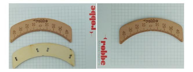
Now glue the plastic holders for the steel wire bracket to the back (super glue). Afterwards the bracket can be clipped into the plastic holders:
