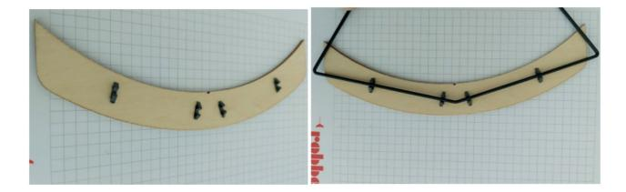
The "suction cup" is guided through the steel wire bracket and fixed with a lock washer. Make sure to use the smaller of the holes in the suction cup! If necessary, widen them slightly with a screwdriver:
