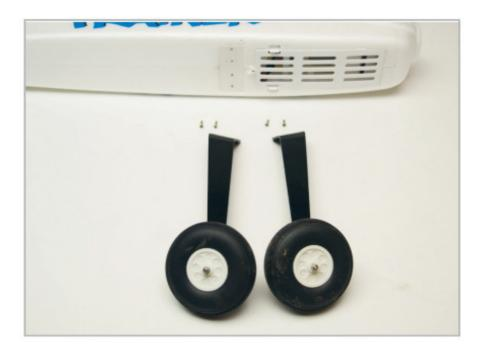
The picture shows the parts required to install the undercarriage.
