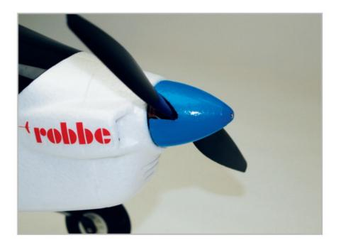
Finally screw the spinner to the propeller driver (see illustration).
