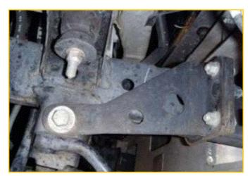
This is the mount from a Genuine Bull Bar. This mount strap uses the bolt hole (below the shock mount) that is required by the tow point. It also conceals the third hole required for correct tow point mounting.
