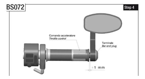
**Warning**: for correct mounting of the right side, check the minimum distance between the bar-end plug and the throttle control (see picture).
