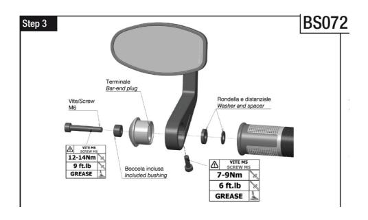
**Attention**: if necessary, use the spacer or washer to adjust the minimum distance between the grip and the terminal.
