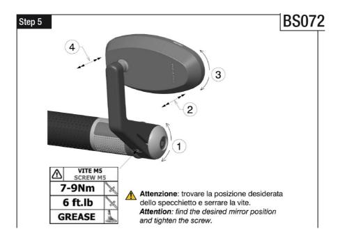
Attention: find the desired mirror position and tighten the screw.
