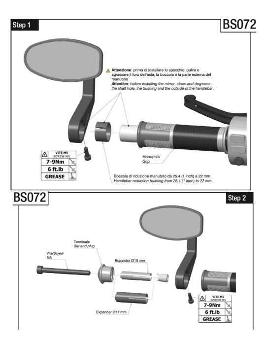
**Attention**: in order to be able to install the mirror with the perforated handlebar, the LP200 expander mounting kit must be purchased. Clean and degrease the mirror shaft hole, the outside of the bar-end plug and the handlebar hole.
