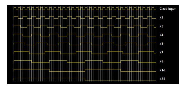
• Diviser outputs 8 different clock divisions. Each output has a 50% duty cycle (equal time spent on and off). Here is a visual representation of the different outputs in relation with the clock input.
