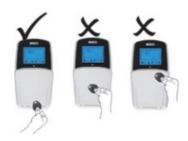
The proximity tag, used with the proximity LCD keypad (RP432 KPP) is correctly used by applying it within a 4 cm distance from the front of the keypad bottom, as shown at right.
