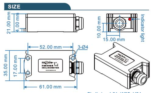
Shell size: L61×W35×H21mm Installation size: L52×W17×H4mm ounting screws: 3 M4 screws
