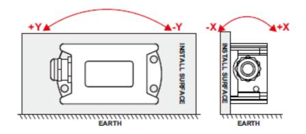
**Remarks**: The factory default installation is horizontal upward, the user can sets the corresponding installation method according to needs, please refer to Article 2 of the operating instructions, and make the corresponding settings.
