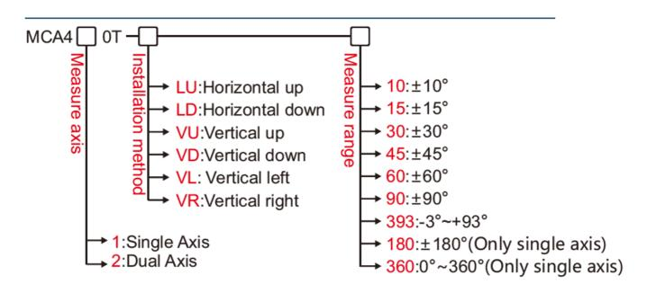
E.g: MCA410T-LU-10: Indicates Single-axis, Horizontal Up Installation Method, ±10° Measure range.
