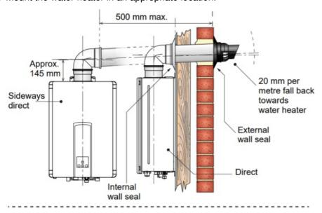
2. Using the dimensions provided, mark a point along the appliance centreline 150 mm from the top of the water heater. This mark forms the centre for the 140 mm diameter wall penetration.
