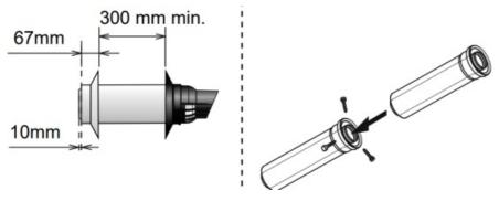
6. Fit the external wall seal to the terminal pipe. Pass the male end of the terminal pipe through the penetration point and weatherproof the penetration. Fit the internal wall seal.
