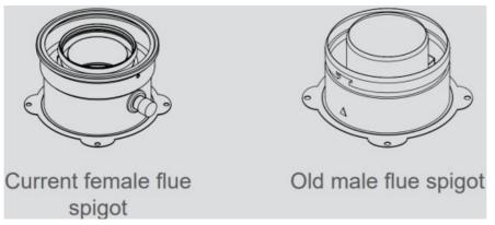
We no longer have male flue spigots that can be retrofitted to our current models.
