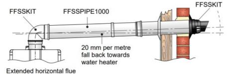
7. Connect the terminal pipe to the bend, ensuring the components are pushed 'fully-home'. Secure the PVC joints of the bend to the terminal pipe with three self-tapping screws (not supplied).
