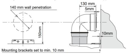
5. Measure the required length for the horizontal terminal to penetrate the wall and allow an extra 67 mm protrusion from the inside wall surface.
