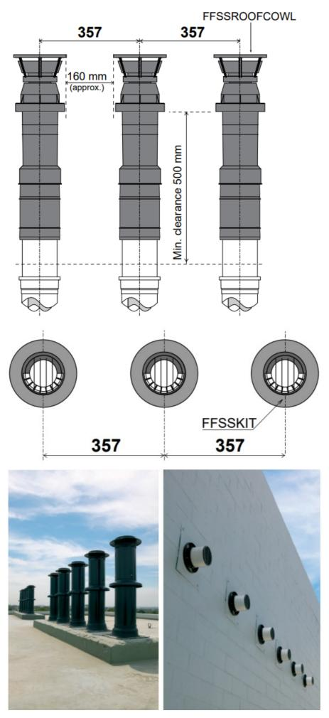
Older style roof cowls and horizontal terminals all terminating at the same height
