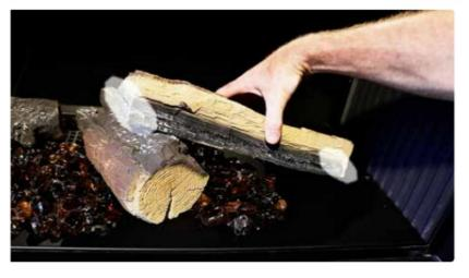
When correctly installed the log should sit evenly on the centre log, with a gap of around 5 mm between the log and the long flame rod to the left of the pilot.
