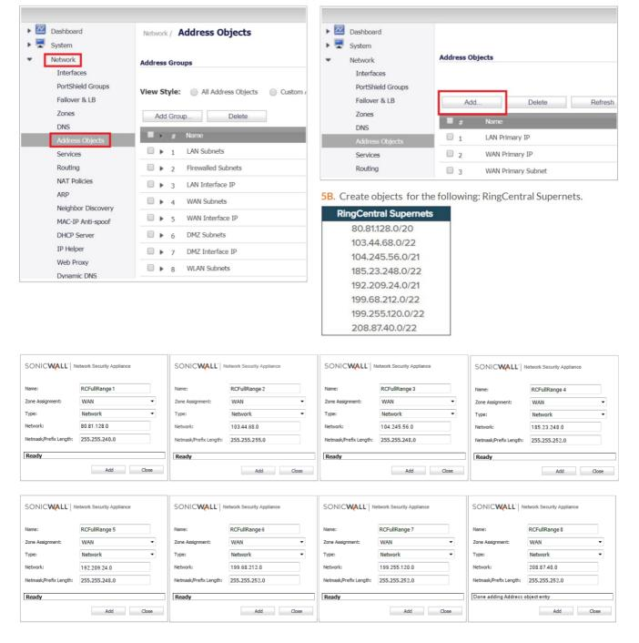
6. A. Once the address objects are added, add the address group from the same section of the interface, as seen below.
